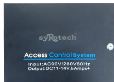
SY-H50 Input : AC90V/260V60Hz Output : DC11-14V, 5Amps+
