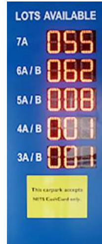
SY-FD11 Display Unit Input Supply : 220V AC Display : 5mm Ultra Bright Communicate : RS 485 Enclosure : MS Powder Coated.
