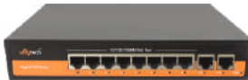
SY-8000P-2T-150W 8*10/100/1000Mbps POE Port +2*10/100/1000Mbps Uplink Port, af/at, 150W POE Power, Extend 250 Meters
